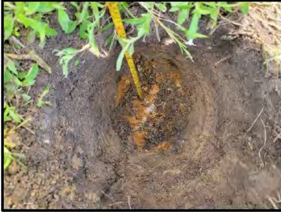
Photo 11. Compacted clay noted in SMF 1A.
