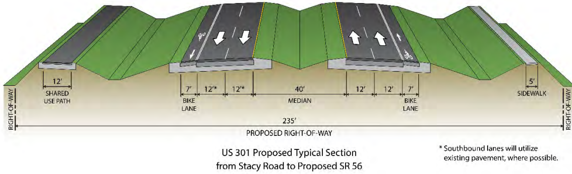
Figure 1.4: Proposed Rural Typical Section
